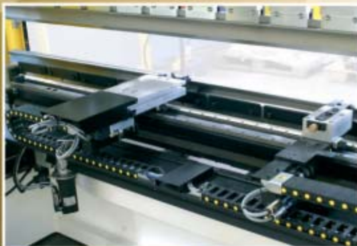
Registro posteriore a 5 assi Five axes backgauge X-R-Z-Z 2 -X 2
