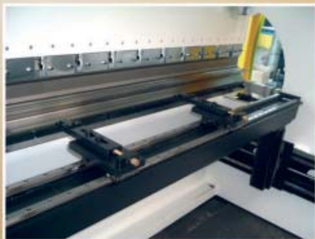
Registro posteriore a 2 assi Two axes backgauge X-R
