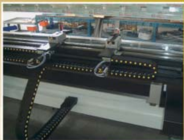
Registro posteriori a 4 assi Four axes backgauge X-R-Z-Z 2
